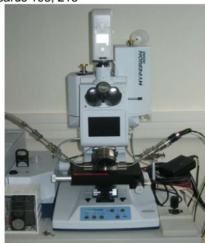
Figure 1: The micro-IR HYPERION and the heating environmental cell used for in situ experiment.
